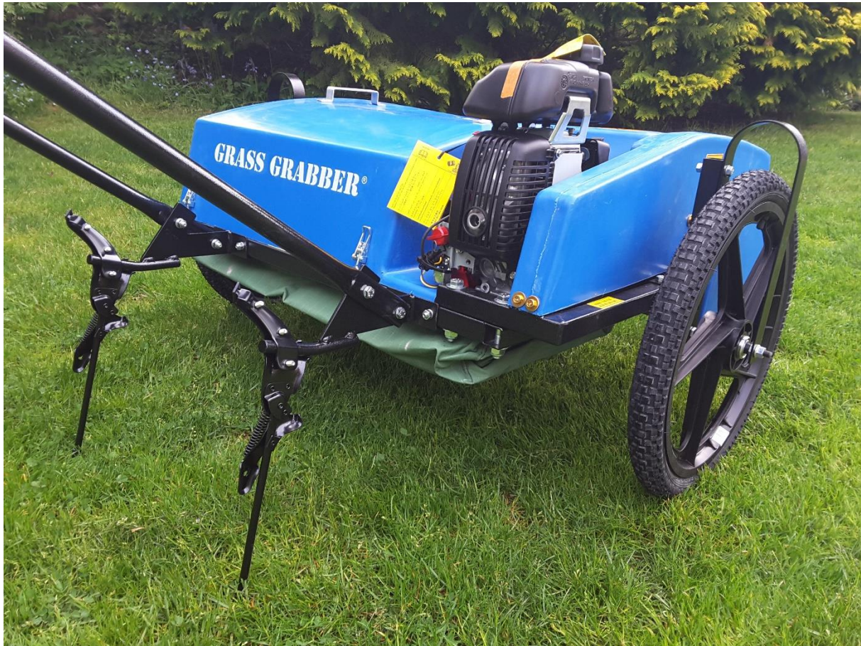
Above: MMG's 'Grass Grabber', a brush seed harvester used at Ragleth meadows
